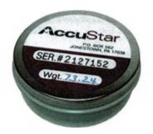
Liquid Scintillation. Liquid scintillation also uses charcoal to measure the radon gas. Instead of measuring the gamma emissions from the exposed charcoal, this method converts the alpha emissions to light, which is then measured.
